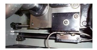
NOTE: START OFF WITH THE READER HEAD POSITIONED MID WAY ON SLOTS.
