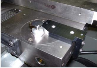
The Microsyn Angle Bracket (4) can now be mounted loosely with the two ¼-20 UNC x 3/8 Socket Button Head Screws (7) and ¼ Flat Washers (6). *(See photograph below)*
