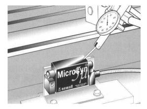
TIP: Check alignment of reader head from the side. It should be parallel to the cross slide. Once again double-check that the set-up tube will fit loosely and freely into the Single End Mounting Bracket.
